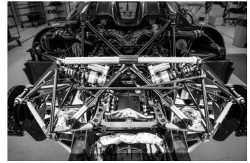
The Triplex rear damper acts against this tendency, providing resistance against 'squat' (both dampers compressing at take-off) but doing nothing during regular single-sided compression of the dampers (e.g. during cornering). The Triplex damper also counteracts the anti-roll bar when driving straight on an uneven road, but does not work against it while cornering. This actually increases comfort and grip.
