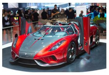
The roof is a one-piece unit made completely from carbonfibre and light enough to be removed by one person. While the design of the roof itself was not a challenge, designing a space for it to fit into the front of the car certainly was.
