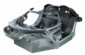
In simple terms, it means that the car is very, very resistant to twisting or flexing when under pressure (e.g. at 2g's in a corner).
