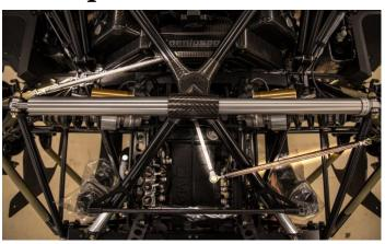
The Z-shaped anti-roll bar on the <u>Agera RS</u> only has one pivot point, instead of the two pivot points on a traditional anti-roll bar. That reduces friction and therefore increases accuracy and response.
