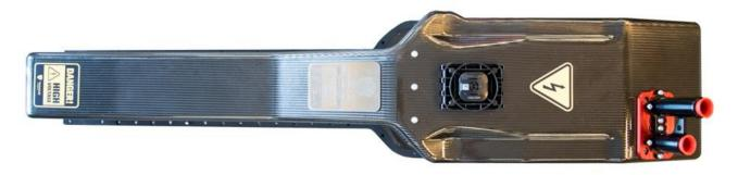
The Regera produces 670 electric hp, and all that from a battery pack that weighs just 66kg with cooling fluids.
