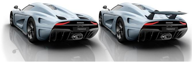
The previous page detailed the benefits of an active rear wing: it provides variable amounts of downforce to optimize performance according to requirements at any given moment – top speed, handling or braking.
