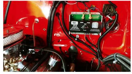
air conditioner. The fan is then forced to run at a set speed in order to get air flow over the A/C condenser coil. In addition to the heavy fan wires, the controller needs a ground, ignition 12V, and constant 12V to provide the various functions, and a safety bypass switch, so there are several wires to be run. But your old fan relay is discarded.
